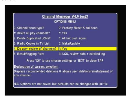
The initial menu allows the basic operation of Channel Manager to be selected –further details of the options and their use is given below. Use the up/down keys to move to the next item, and left/right to change setting for the current selection. More information is given on the current selection at the bottom of the screen. More details of the options available without the ".ini" file are given below. When you are satisfied with the selections, press "OK".
